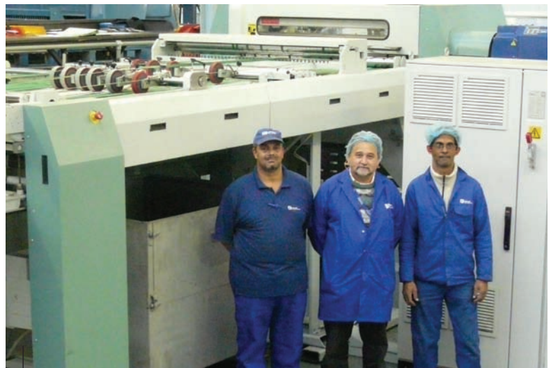
The SHM 1450 sheeter attains speeds of 335m/min, with a maximum sheet width of 1 450mm. Size or format changes can take less than 10 minutes, including loading a new roll. It also features non-stop operation and automatic pallet change. All these features add up to an easier life for the operators.
