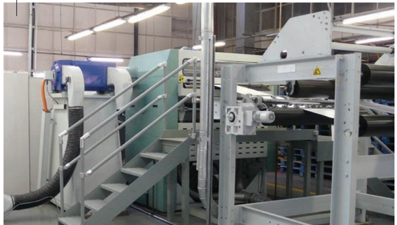
The SHM 1450 sheeter attains speeds of 335m/min, with a maximum sheet width of 1 450mm. Size or format changes can take less than 10 minutes, including loading a new roll. It also features non-stop operation and automatic pallet change. All these features add up to an easier life for the operators.
