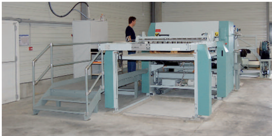
The new Pemco SHM 1450 sheeter is able to cut rigid and impact resistable films
