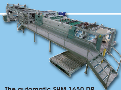
The automatic SHM 1650 DR folio-size sheeter offers a good clean cut with minimal waste
