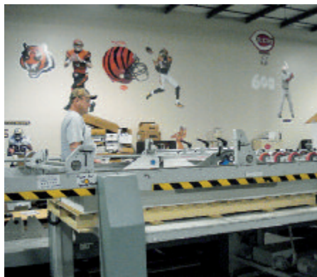
SHM 1450 SR sheeter installed at DCM to sheet repositionable vinyl
